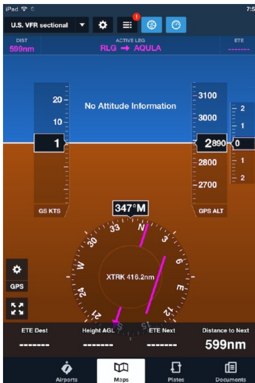
Attitude Indicator with GPS input but no SV subscription or AHRS input.
